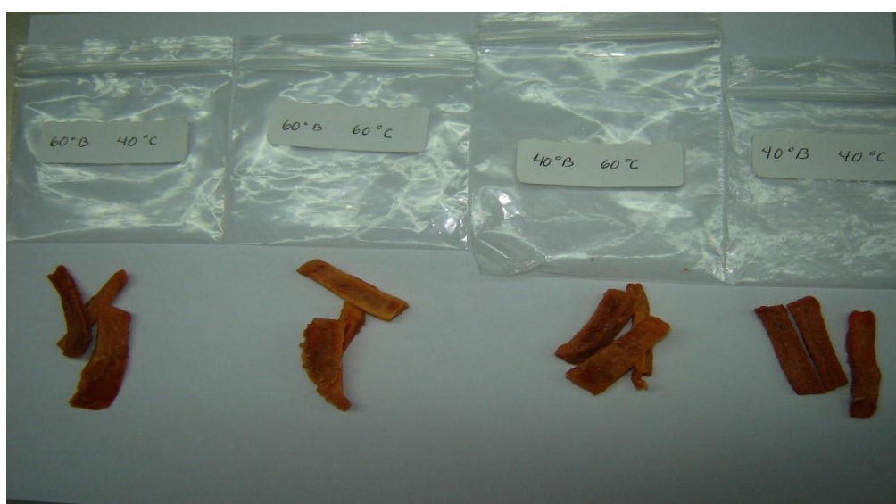
Figure 5. Mamey samples osmotically dehydrated at 40 and 60 ° Brix and air dried at 60 and 40 °C
