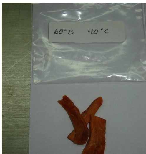
Figure 3. Samples of Mamey osmotically dehydrated at 60° Brix and air dried at 40 °C
